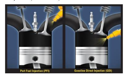
This allows for a more even burn of the fuel, the intent being, added power and greater MPG.
